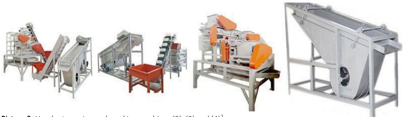
Picture 3: Hazelnut gauging and cracking machines (2), (3) and (4) 2
